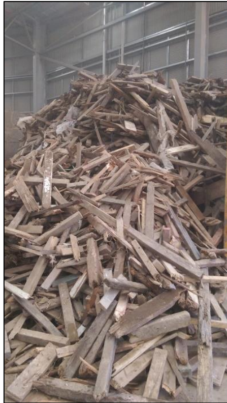
Figure 2 – Sorted timber waste at a waste management facility awaiting collection.
